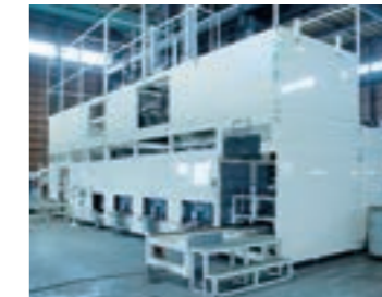
A cleaning machine for degreasing, washing, and drying of finely broken titanium scrap (Naoetsu Plant, Showa Metal Co., Ltd.)
